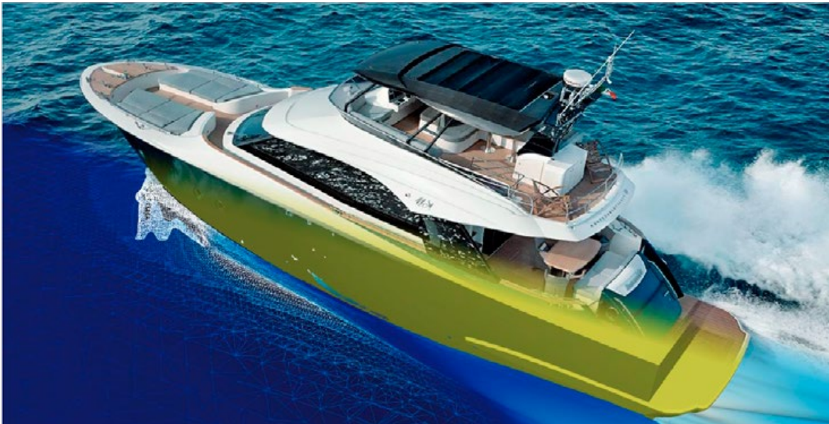
A rendering of the CFD simulation results superimposed to the actual wave pattern past a yacht advancing in non calm sea conditions.
